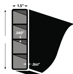
We crimp or notch both sides on both ends to secure the rail into the post. The triple-rib rail design provides extra impact resistance while maintaining flexibility for the safety of your horses.
