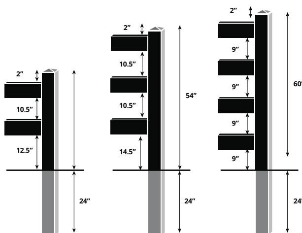
Rails are 16' long and designed to alternate between posts to increase strength. Posts are placed on 8' centers. **Call for more information on spacing and sizes.**
